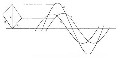
FIG. 48. Diagram representing the addition of sine waves.
